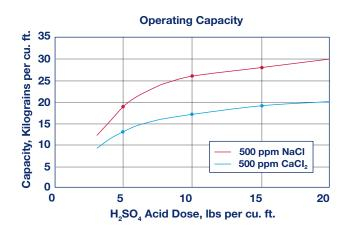
Capacity based on 500 ppm of stated salt (as CaCO<sub>3</sub>) with 0% alkalinity, 36 in. bed depth, flow rate of 2 to 4 gpm per cu. ft. and >30 min. chemical injection time. Sulfuric acid concentration must be stepwise when calcium concentration exceeds 20% of total cations. No engineering cowngrade has been applied.
