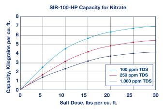
Capacity and leakage based on 10% NO3 and 40% SO4 in the feed and 35.7 ppm NO3 endpoint (all as CaCO3). Capacity and leakage are for nitrate alone. TDS is for total anions
